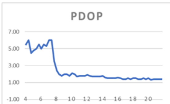
Fig. 11. PDOP coefficients on different number of satellites
