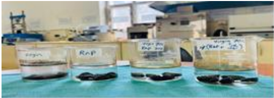
Figure 5: Loose mix of the four types of mixes
