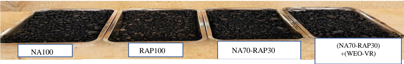
Figure 5: Loose mix of the four types of mixes
