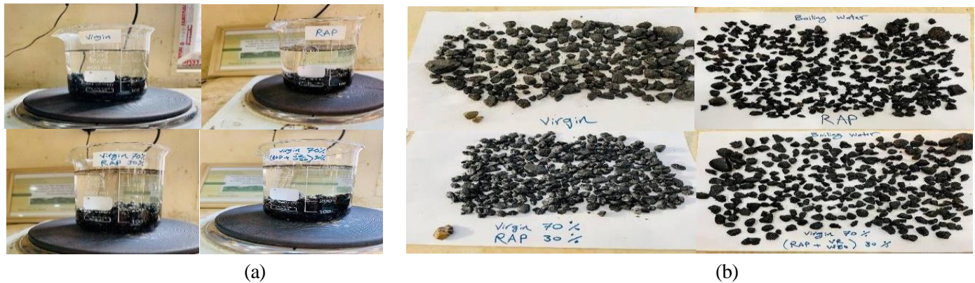
Figure 9: Boiling water test, (a) samples on the heater, (b) samples after test
